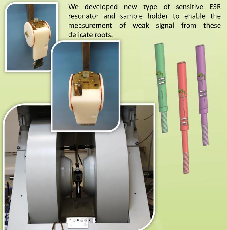
We developed new type of sensitive ESR resonator and sample holder to enable the measurement of weak signal from these delicate roots.
